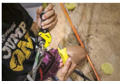
1 Insert the Self Belay key in the device all the way in.
