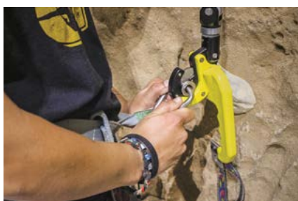
1 Insert the Harness Piece in the Self Belay all the way down until it clicks.
